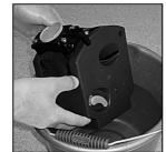
Remove the B2C coffee chute assembly. Unscrew the two knurled thumbscrews and remove the coffee chute and coffee chute cover.
