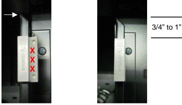
**Step 2 – Magnetic Switch:** Peel off the tape backing on the switch leaving the side screw plastic piece intact. Locate the switch on the door baffle as shown below with the right edge against the metal edge fold. Insure that the height of the switch is the same as the magnet.
