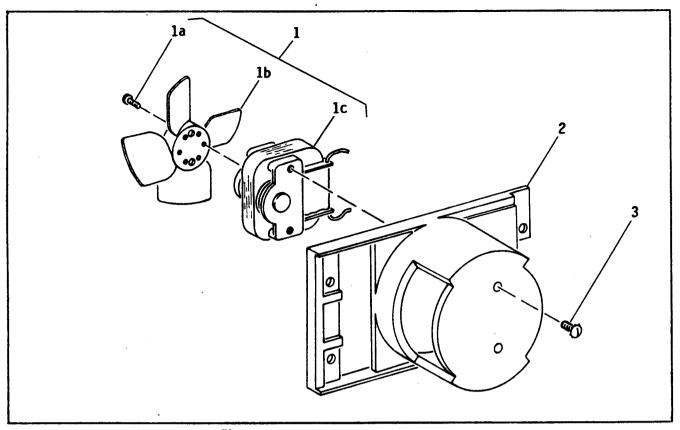
Figure 4-6. Fan and Housing Assembly
