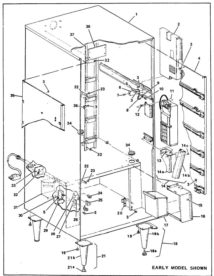
Figure 4-2. Cabinet Assembly (1 of 3)
