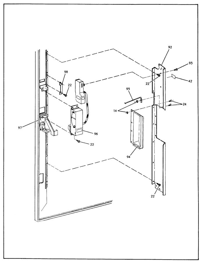
Figure 4-7. Door Assembly, Final (3 of 5)
