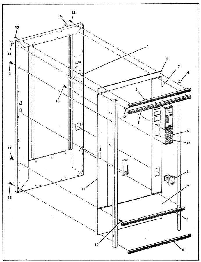
Figure 4-7. Door Assembly, Final (1 of 5)
