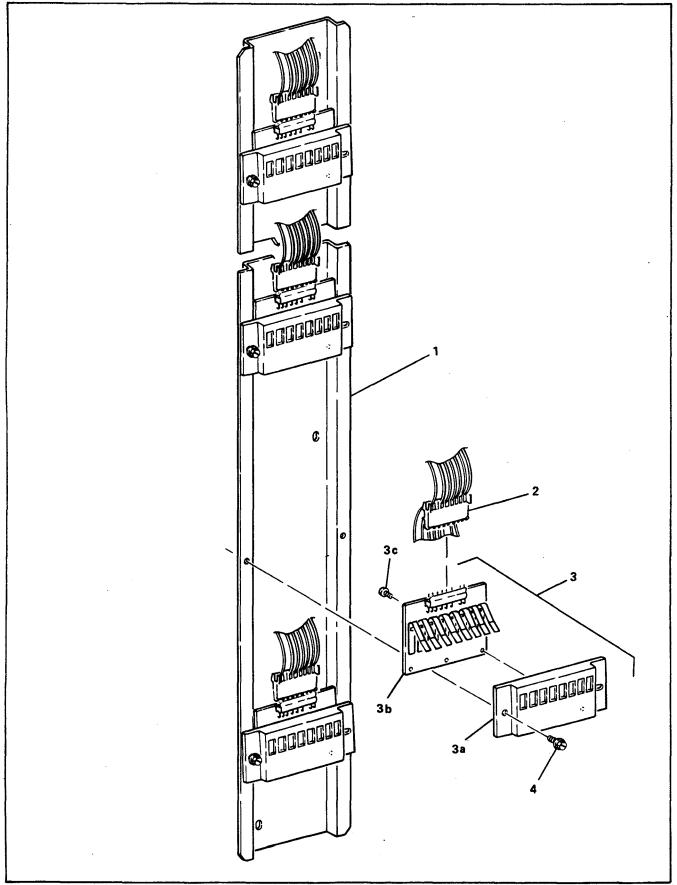
Figure 4-5. Channel and Receptacle Block Assembly
