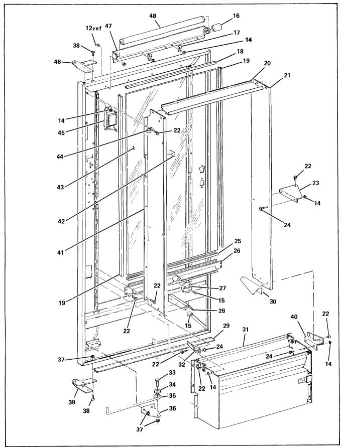
Figure 4-7. Door Assembly, Final (4 of 5)
