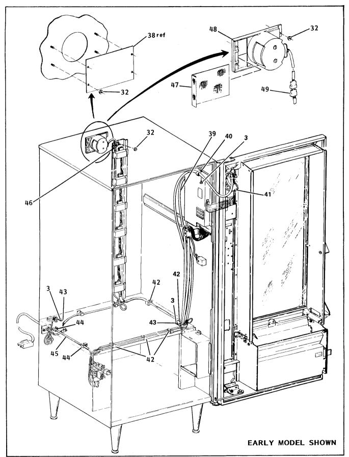
Figure 4-2. Cabinet Assembly (2 of 3)
