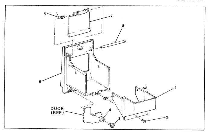
Figure 4-9. Coin Receptacle Assembly
