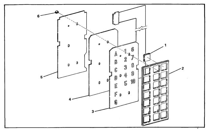
Figure 4-8. Push-Button Grid Assembly
