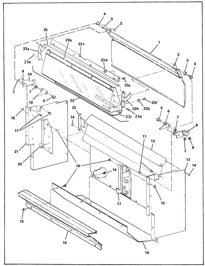
Figure 4-10. Delivery Pan Assembly
