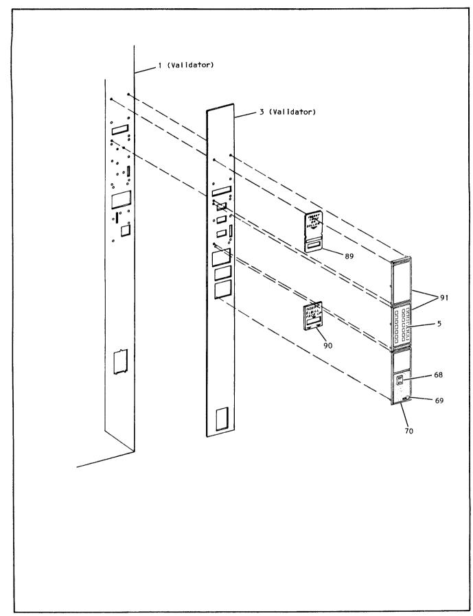
Figure 4-7. Door Assembly, Final (2 of 5)
