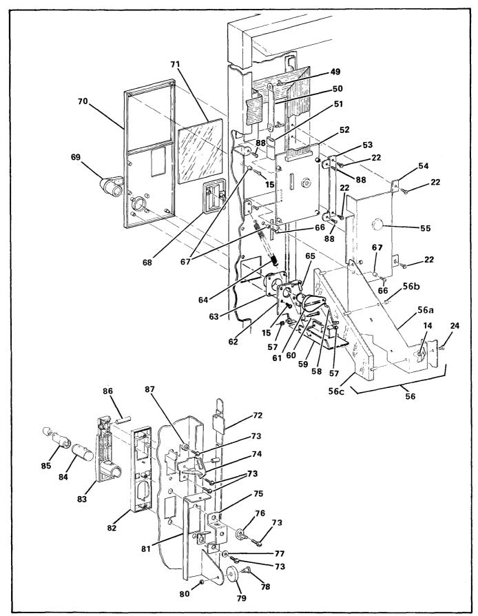
Figure 4-7. Door Assembly, Final (5 of 5)
