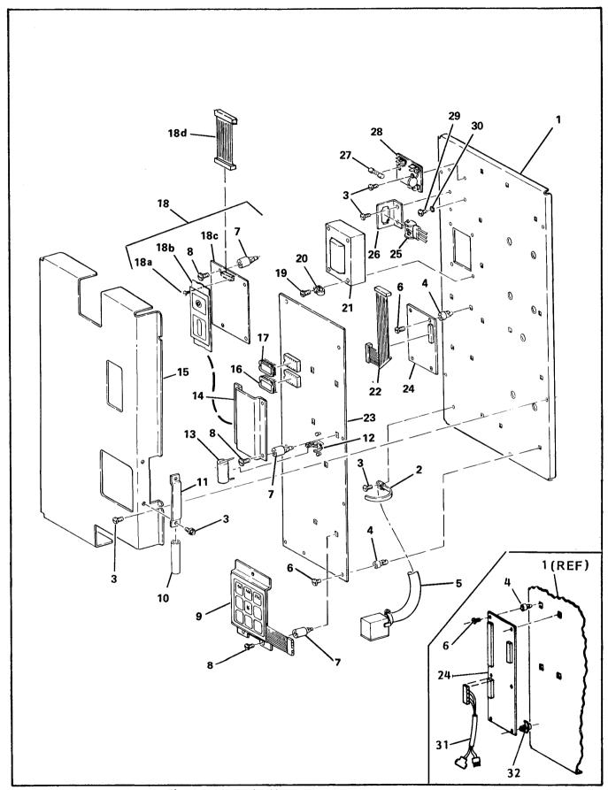
Figure 4-3. Controller PCB and Component Assembly
