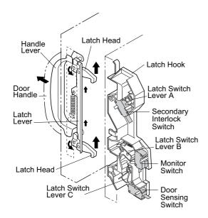
Figure D-1. Door Open Mechanism.
