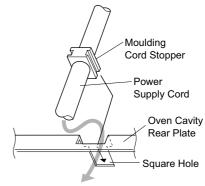
Figure C-3b. Power Supply Cord Replacement
