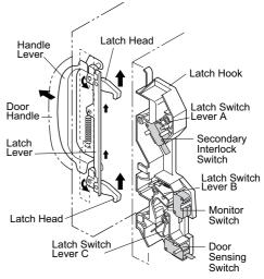
Figure C-5. Latch Switch Adjustments
