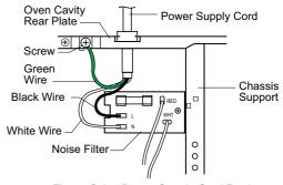
Figure C-3a. Power Supply Cord Replacement
