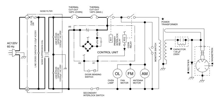
Figure O-1. Oven Schematic-Off Condition
