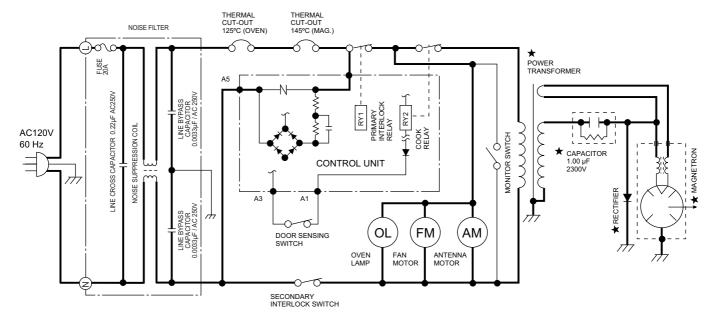
Figure O-2. Oven Schematic-Cooking Condition
