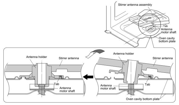
Figure C-10. Stirrer Antenna Assembly Installation
