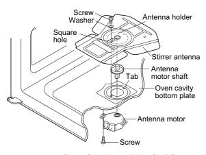
Figure C-8. Antenna Motor Shaft Removal
