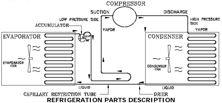
The Compressor, Condenser, Drier, Capillary Tube, Evaporator, and Accumulator are part of a sealed system (refer to figure 16). These items are not available separately. For the part number of the sealed refrigeration system refer to the common parts section of the manual.
