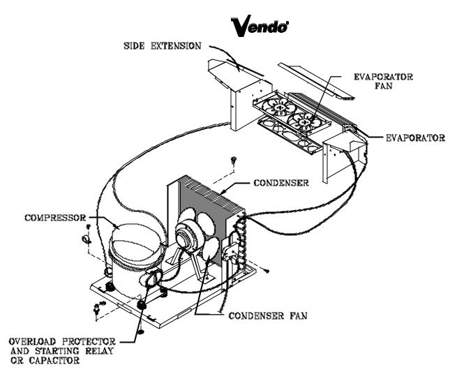
(The parts listed below are not part of the sealed refrigeration system and are available separately. For part numbers, see the refrigeration assembly in the common parts section of the manual.)
