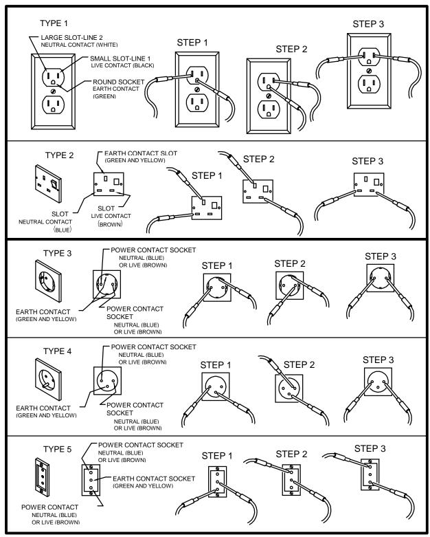
FIGURE 1 CHECKING FOR PROPER POLARIZATION
