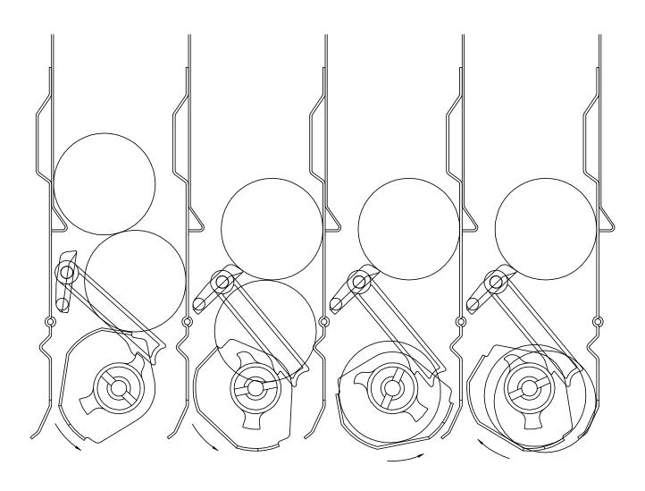
BUCKET ROTATES COUNTERCLOCKWISE CAM PUSHES LINK LINK OPENS GATE BUCKET CONTINUES COUNTERCLOCKWISE GATE CLOSES AS PRODUCT LOWERS INTO BUCKET BUCKET REACHES
