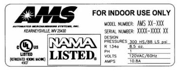
Figure 1. Example of Serial Plate
