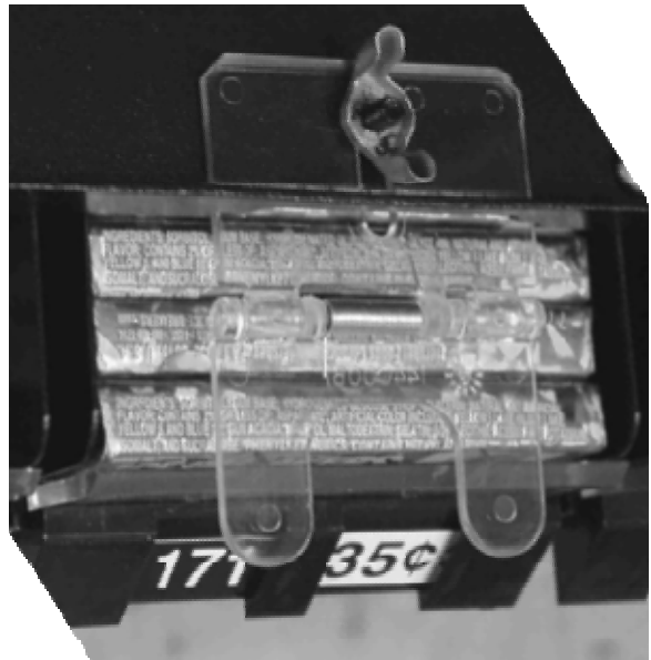
Figure 10: Correct gum and mint adjustment.
