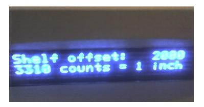
Type in a higher number to raise the picker and a lower number to drop the picker, The top of the picker should strike the target no higher than  $1/16^{th}$  from the top ( do not hit shelf) and no lower than half way down.
