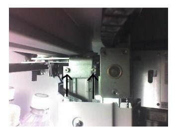
3) Check gates for cracks:
