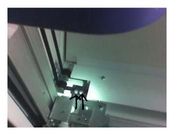
Loosen the 2 screws below the picker cup and pivot the bottom of the "Y" axis left or right until the bottom gap is the same distance from the wall as the top gap.
